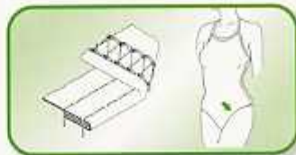
Top Stitching on Pre-attached Elastic tape
