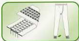
4 Needle Joining Seam
